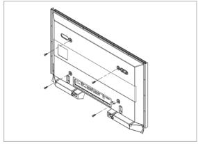
4. Remove safety pin (3) and insert the 4 product holders into the corresponding bracket holes (1). Then place the product(2) so that it is firmly fixed to the bracket. Make sure to re-insert and tighten the safety pin (3) to securely hold the product to the bracket.
